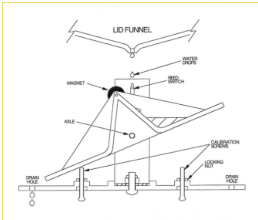
Figure 1. In a tipping bucket apparatus, rainfall is gathered in the funnel-bottomed lid and dripped into one of two buckets. When the required water volume is reached, the bucket falls and empties. The action moves the other bucket into position to repeat the process.
