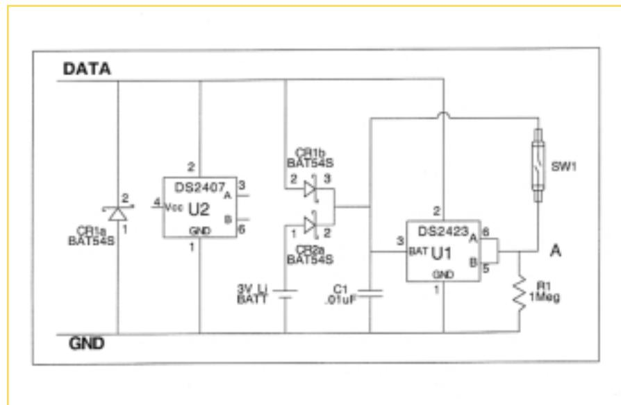
Figure 2. A magnet on the tipping bucket mechanism momentarily closes the magnetic reed switch each time a bucket tips and empties. This increments the DS2423 digital counter one count. Power for the counter is normally supplied by CR1b and C1. Lithium battery backup can be added using CR2a to allow rainfall to be recorded even when the bus master is off-line.
