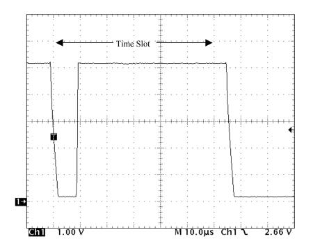
This image shows a "Read One" or "Write One" time slot. The master pulls the bus low for about  $10\mu s$  and then releases it. Note the slew-rate controlled fall time. The time slot lasts for about  $70\mu s$ , after which another time slot occurs. Note that the time base is changed to  $10\mu s$  per division.
