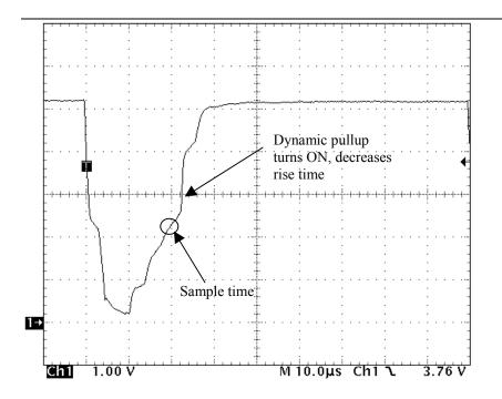
A more advanced network bus driver uses impedance matching and dynamic pullup to overcome the added weight of the long network and slave devices. This waveform shows a Read or Write One time slot and the action of the dynamic pullup.
