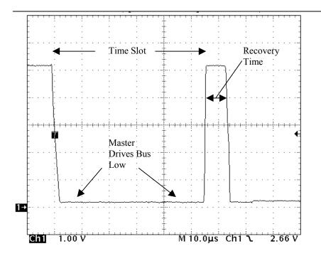
This image shows a "Write Zero" time slot. The master pulls the bus low for 60µs and then releases it for about 10µs before another time slot begins.
