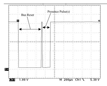
This image also shows a bus reset/presence sequence. The master pulls the bus low for 480µs, which is longer than any time slot can hold the bus low. All the devices on the bus recognize this as a reset operation. slave devices respond to a bus reset by issuing a presence pulse. Multiple slaves will generate their presence pulses during the same period, and they will overlap to form a single pulse. (Note that the time base is 200µs per division.)
