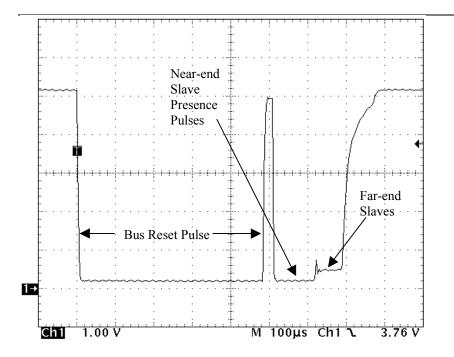
During bus reset sequences, the dynamic pullup is used to overcome the network weight after the reset pulse, and then again after the end of the presence pulse(s). In this image, the overlap of near- and far-end presence pulses can be observed. The added resistance of the cable between the master and the far-end slave causes the low level to be higher for far-end devices than for near-end devices.
