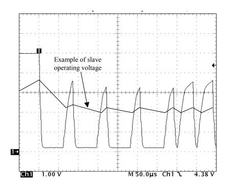
When rise time is insufficient, recovery time (the period between time slots) may be insufficient to allow the bus to reach a level sufficient to recharge the slave devices. In the image above, the average DC level that the slaves have to work with has become dangerously low. Slaves may reset due to power starvation, especially during long strings of Write Zero time slots.
