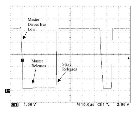
This image shows a "Read Zero" time slot. The master pulls the bus low for about  $10\mu$ s and then releases it. However, a slave device is returning a zero bit by holding the bus low for a longer time. The slave device time base may vary between  $22\mu$ s and  $60\mu$ s. The master samples the bus at  $20\mu$ s and so reads a zero bit in this example.
